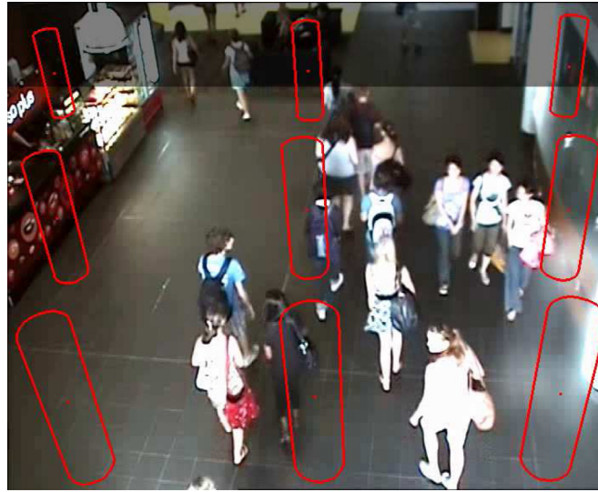
(a) Camera 3. A camera calibration technique [23] is used to project a prototypical human-sized cylindrical object into the scene at any location. This hypothetical cylinder model is used to construct the density map S(i, j) at every pixel (Equation 1). The density map is used to normalise features to achieve scene invariance. Only a sparse subset of the cylinder models are shown here; however, the system constructs them around every pixel (during initialisation of the system only).
